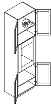
**Step 3:** slide the back panel into its slot in the top and bottom panels.
