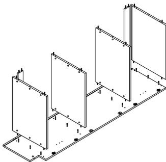
**Step 5:** Install the 3/4" overlay soft-close hinges in the upper holes of the doors; Install the 3/4" overlay 6-way hinges in the lower holes of the doors. Install the male fasteners on the center frame.
