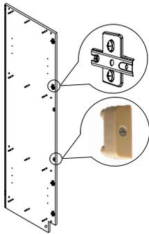
**Step 4:** Install the other side panel and toe kick using cam locks and wood dowels.
