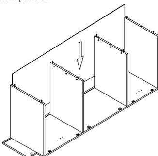
**Step 8:** Adjust the hinges to ensure that the clearance for all doors is the same. Finally, check the firmness and stability of the cabinet tightening the cam locks as necessary.
