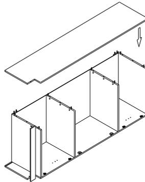
**Step 6:** Connect the doors to the box, hinges on the door panels snap into the hinges on the side panels. Insert the male fasteners into the female fasteners to attach the center frame.
