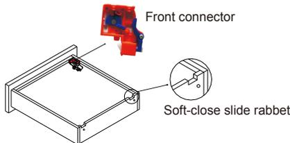
**Step 5:** Install the drawers. First, extend the arms of the drawer slides and place drawer on top of the extended arms. There is a notch cut into the bottom of each side of the drawer where the arms rest. Reach under and pull the arms to meet the drawer front connector. The arms should slide forward until a "click" is felt. This is a secure connection. After that, a small lever on the drawer front connector can be used to make small adjustments to correct clearance.
