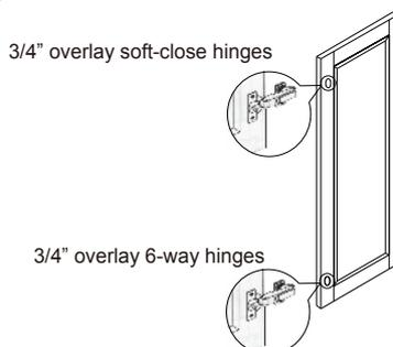
**Step 7:** Connect the doors to the box, hinges on the door panels snap into the hinges on the side panels.
