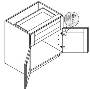
**Step 8:** Install the shelf supports at the desired height then place shelves on top of the supports. Adjust the hinges to ensure that the clearance for all doors is the same. Finally, check the firmness and stability of the cabinet tightening the cam locks as necessary.
