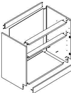
**Step 3:** Attach the Undermount soft-close slides onto the side panels using the pre-drilled holes and the nickel round screws.
