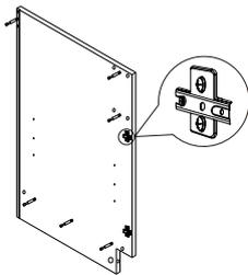
**Step 2:** Assemble the cabinet using cam locks and wood dowels. Start by screwing in all the male ends of the cam locks and inserting the wooden dowels. When the sides, bottom base and braces are loosely connected, tighten everything with the female part of the cam locks. Finish by sliding the back panels into its groove.
